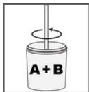
1. Before mixing Parts A and B together, thoroughly mix Part B in a clean pail with a low-speed drill (400 – 600 rpm) that has a paddle attachment.
