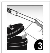
3. Dispense the initial amount of material from the mixing nozzle onto a disposable surface until the product is a uniform gray color with no streaks. Adhesive must be properly mixed in order to perform as published. Dispose of the initial amount of adhesive according to federal, state and local regulations.
