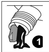
1. Remove the protective cap from the adhesive cartridge and insert the cartridge into the recommended dispensing tool. Before attaching the mixing nozzle, balance the cartridge by dispensing a small amount of material until both components are flowing evenly.
