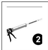
2. Screw on the mixing nozzle supplied with the cartridge after properly balancing the cartridge. Do not modify mixing nozzle. Confirm that the internal mixing element is in place prior to dispensing adhesive. Take note of the air and base material temperatures and review the working/full cure time prior to injection.
